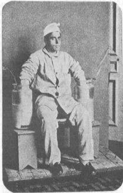
Figure 11. Patient attached to Einthoven's string galvanometer. Reprinted from W. Einthoven, "Le Télécardiogramme," Archives Internationales de Physiologie , vol. 4 (1906-07), p. 143.
